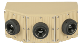
3 x 40° x 30° FOV electronically stitched to provide seamless 107 x 30 video
